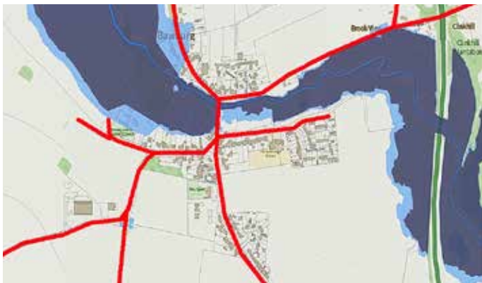
Flood-plain analysis at Bawburgh on the Yare, showing the narrowing of the flood plain at the crossing point
