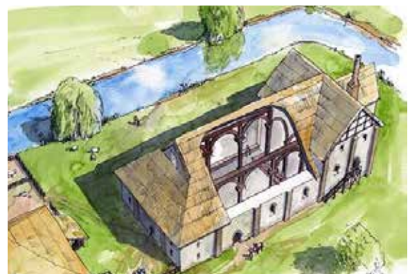
Aisled Hall at Weeting Castle Cut away drawing from English Heritage website.
