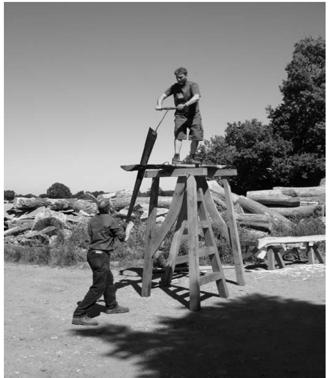
Andrew (under dog) and Rick (top dog) using saw with great skill on a high trestle in the place of a saw pit.
