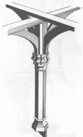
right: The similar crown post from the Woolpack, Coggeshall (illustration from Hewett, C., English Historic Carpentry, p308)
