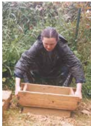
Making clay lump in 2001, guided throughout by Richard Hyde - Diana and ? making clay lump
