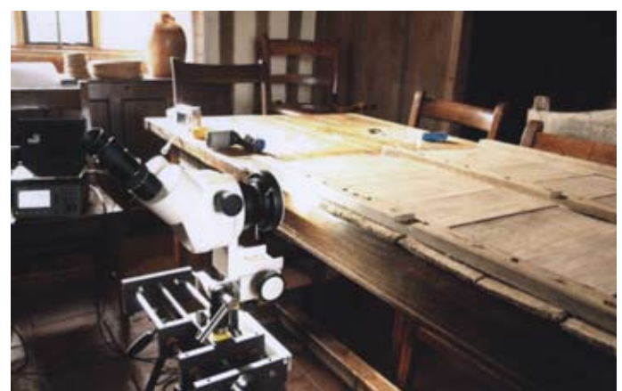
Photo 3 Dendro dating shutters using the technique usually employed for paintings on panels Manor Farm, Pulham Market.
