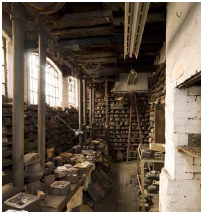
Figure 1 - one of the stamp shops, with drop stamps and dies (All photos provided by the author)
