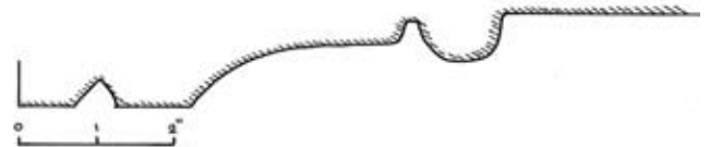
CHAMFER STOP PRINCIPAL JOIST WEST X-WING TACOLNESTON HALL, TACOLNESTON SURVEYED BY: MASH, M. BROWN, S. BROWN, L. HODGE & K. MACKIE DRAWN BY SUSAN J. BROWN FULL SIZE MAY 2008
