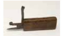
race knife with compass point for drawing circles
